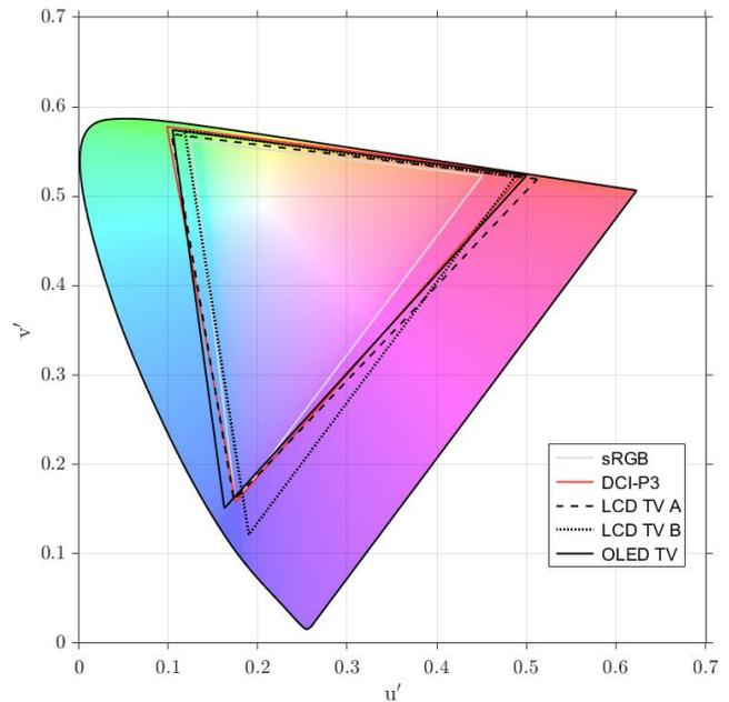
**Figure 1.** The color gamuts of the three test displays as well as sRGB and DCI-P3 for comparisons at CIE1976  $u'v'$  diagram
