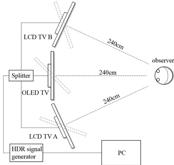
**Figure 2.** The experimental setup (top view)
